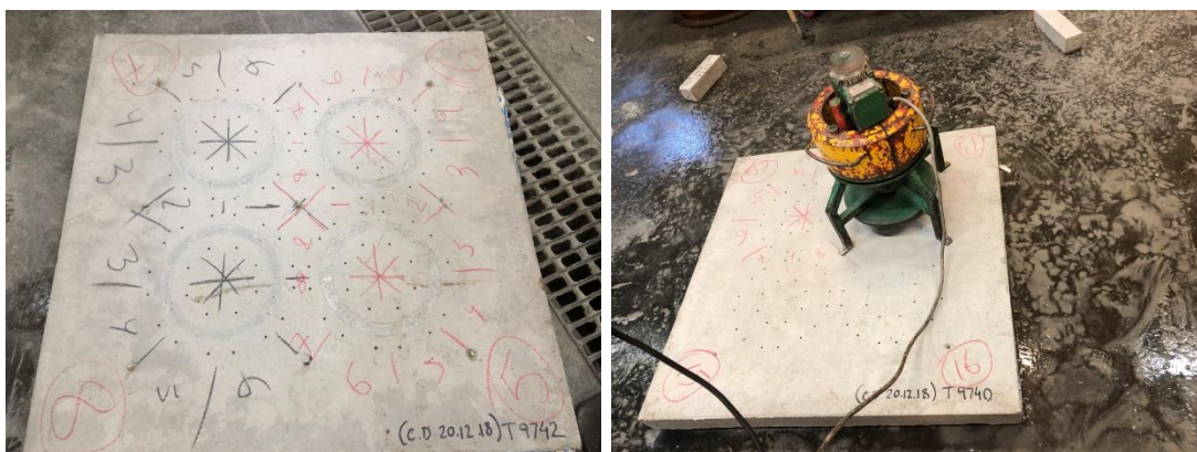
Figure 7: Abrasion resistance test sample and equipment
