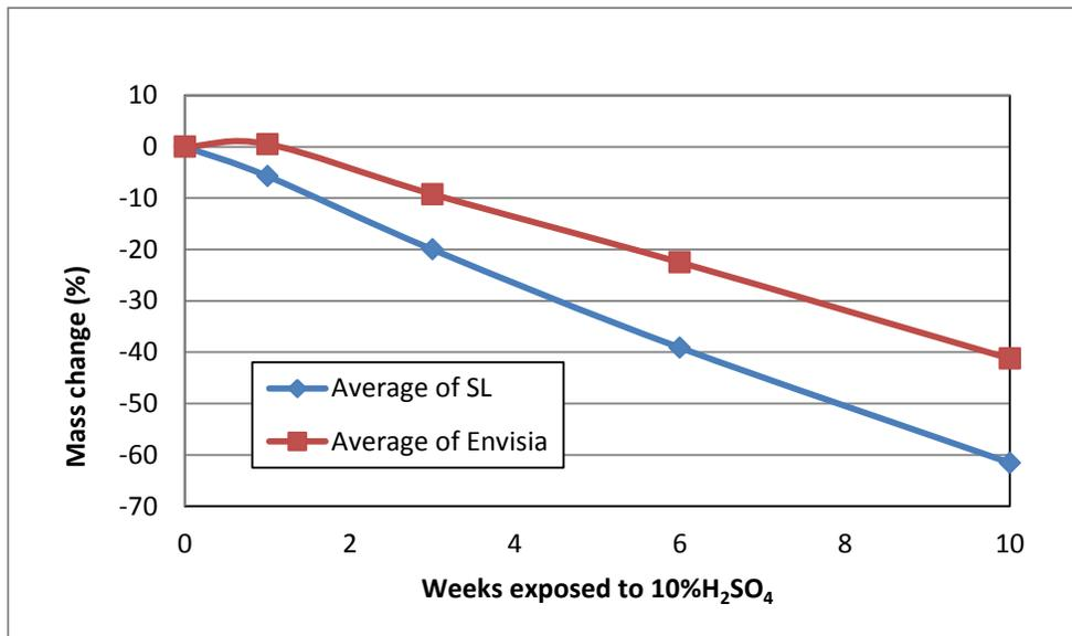
Figure 2. Mass change of Envisia® and SL concretes after 10% H<sub>2</sub>SO<sub>4</sub> exposure.
