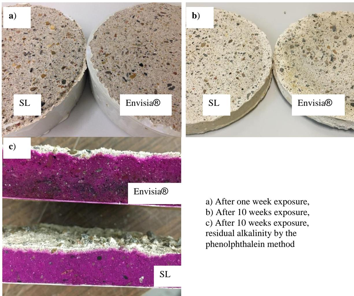
Figure 3. Images of Envisia® and SL mortar specimens after 10% H<sub>2</sub>SO<sub>4</sub> exposure.
