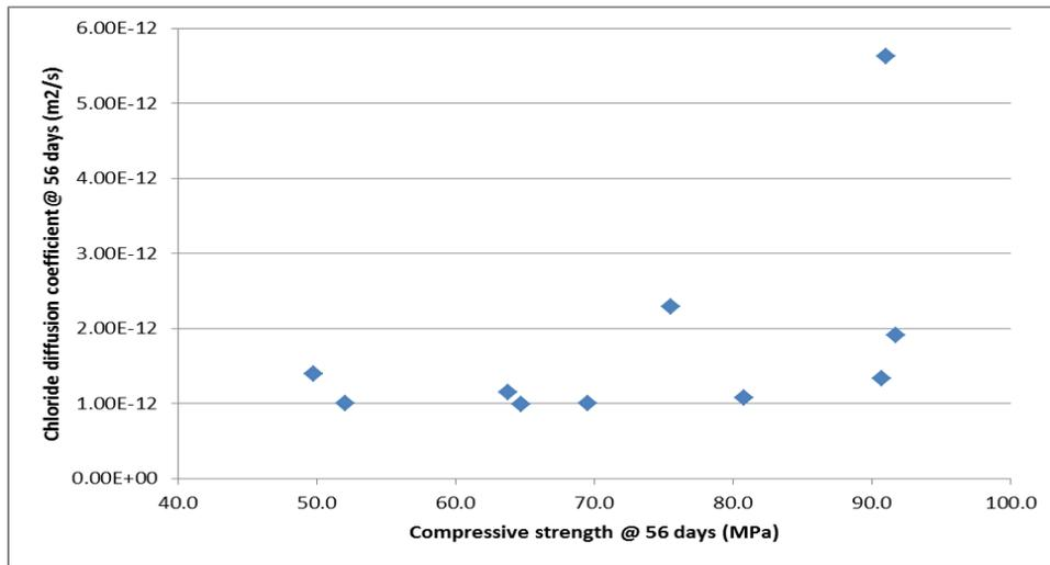
Figure 1. CDC at 56 days curing vs Compressive strength at same age
