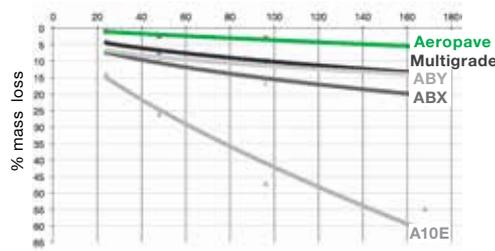
Fig2. Evaluation of Asphalt Fuel Resistance
