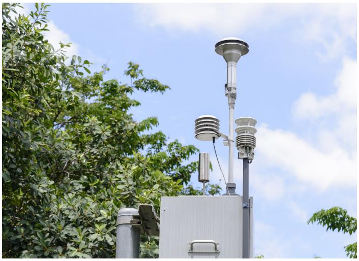
Example of air pollution detectors used for measuring air quality
