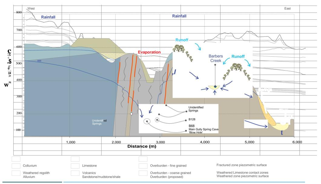
Simplified hydrogeological conceptual W-E cross-section
