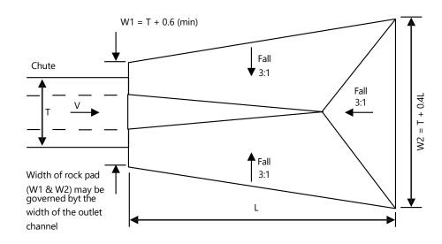
T = Maximum top width of flow at the base of chute
