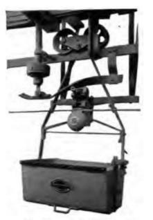
Fig. 9. Carrier, with Webber Patent Compression Grip, showing Patent Automatic Attacher.
