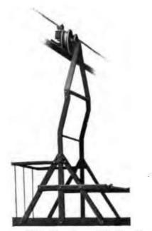
Fig. 11. Bale Carrier, with Overhead Grip.
