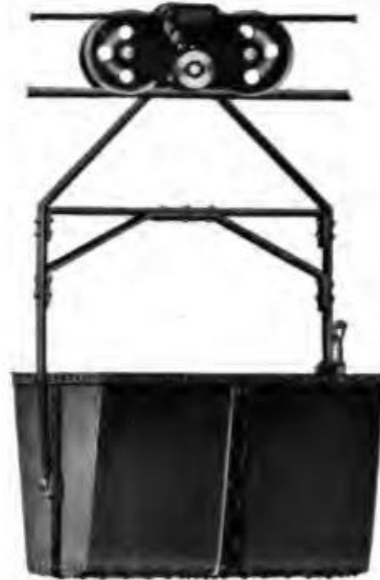
Fig. 10. Carrier, with Bleichert Patent Automatic Overhead Grip.
