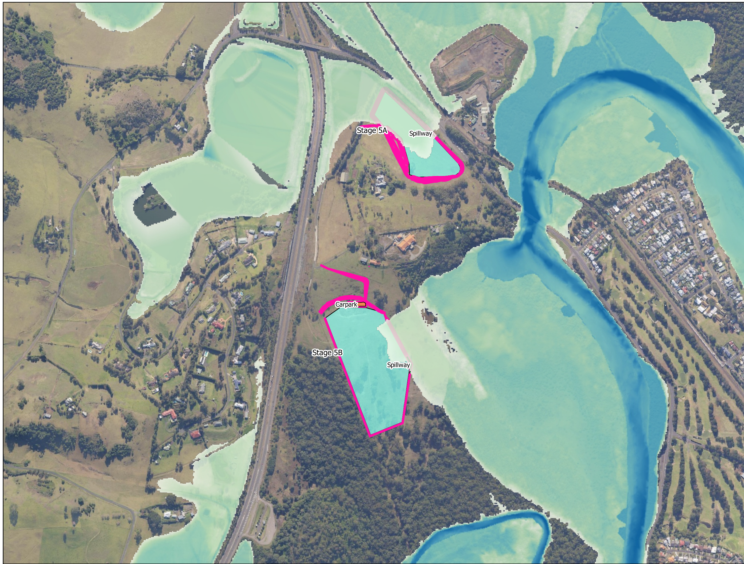
FIG 6. 20y ARI Flood depth, existing conditions.
