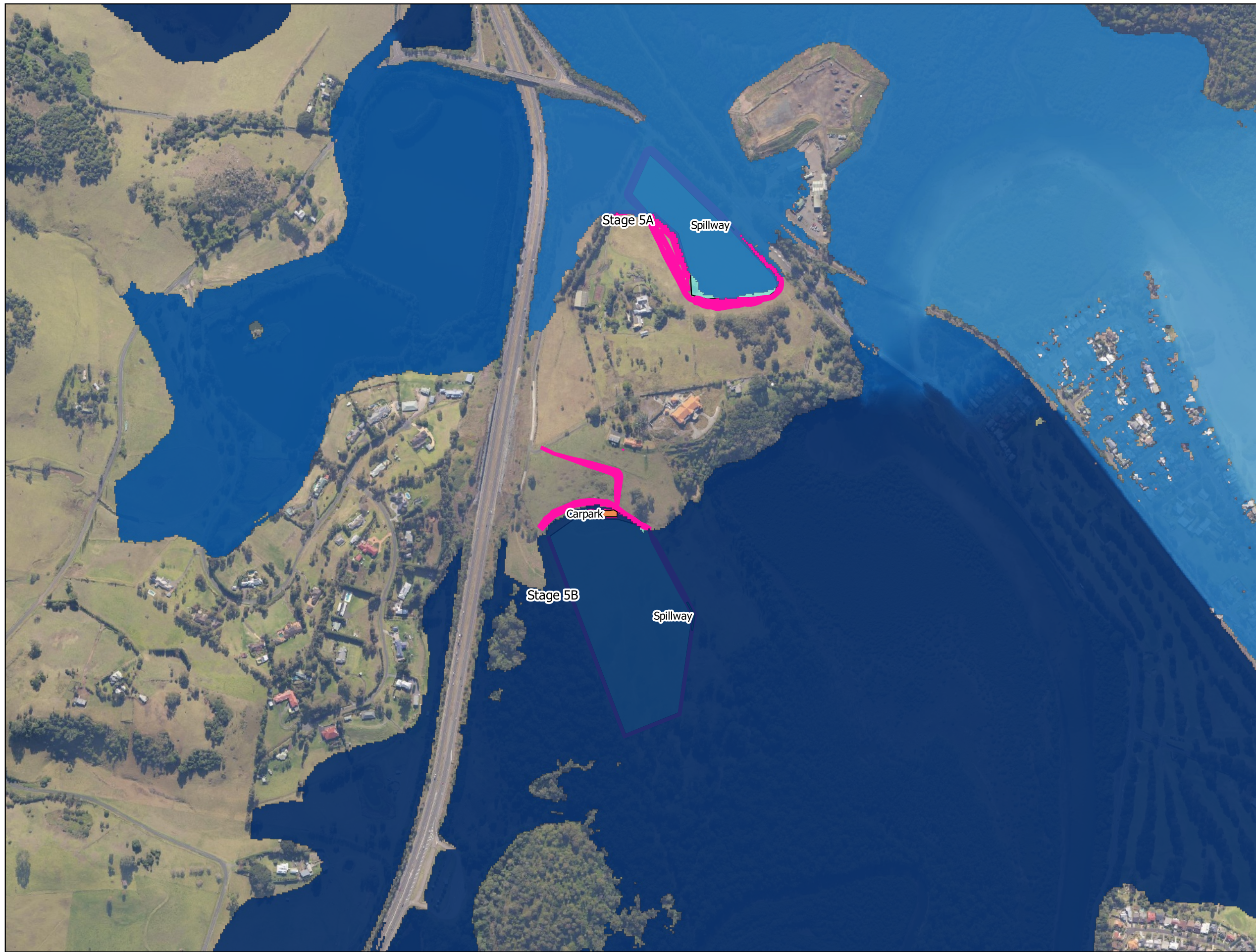
FIG 28. PMF Flood height, proposed conditions.
