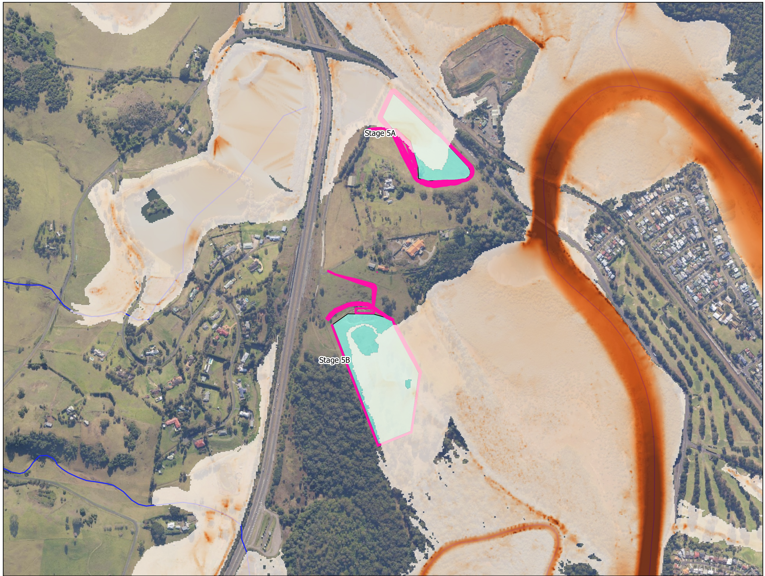
FIG 3. 100y ARI Max velocity, existing conditions. 18/07/2019
