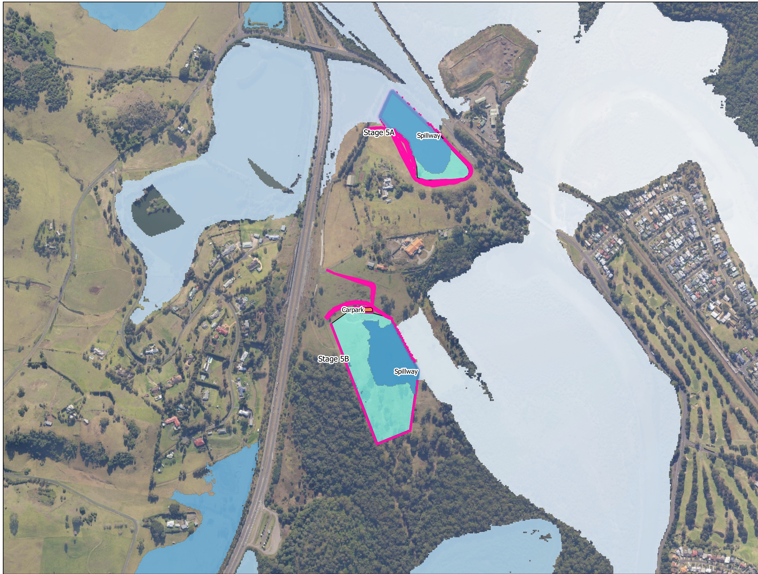
FIG 25. 5y ARI Flood height, proposed conditions.
