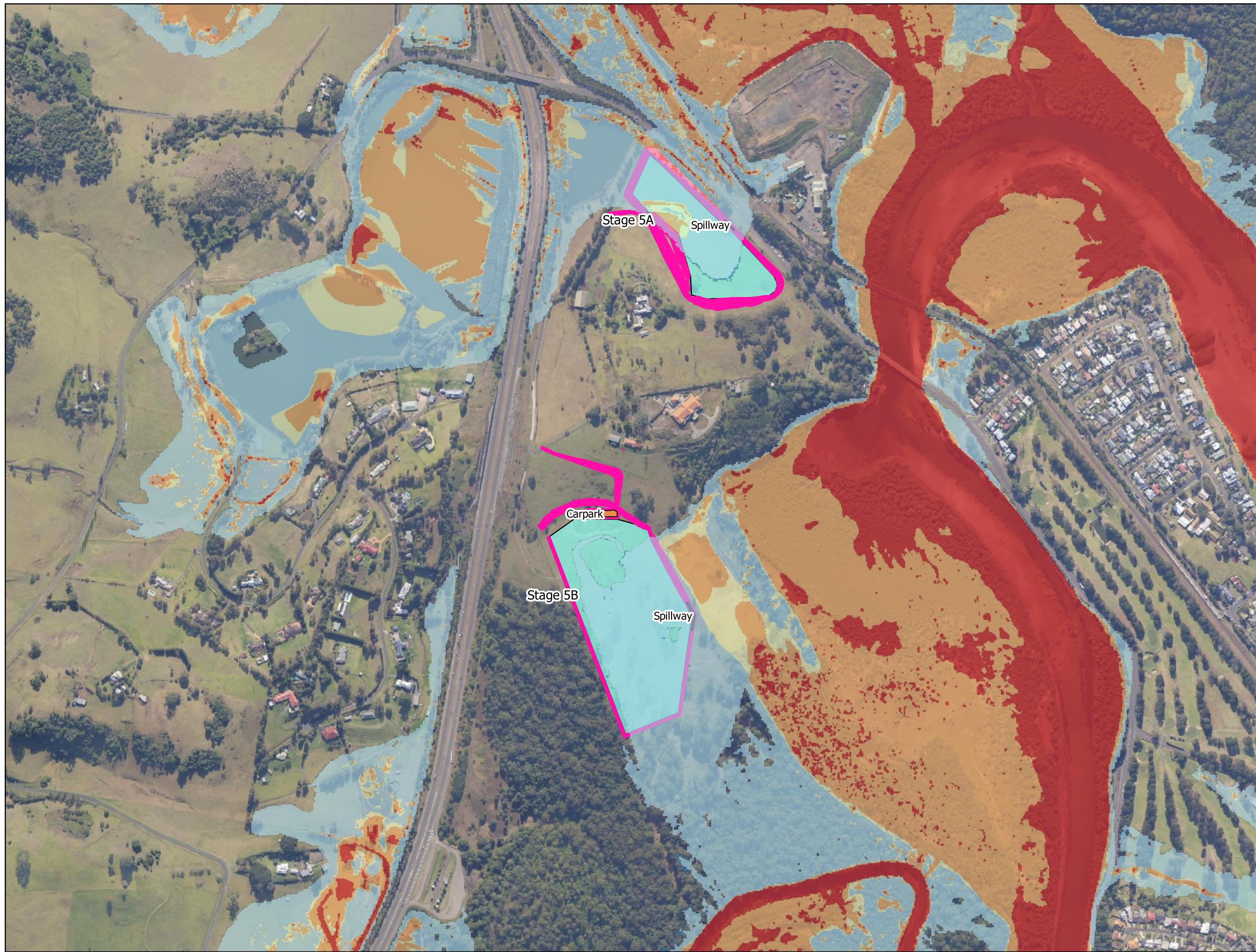
FIG 13. 100y ARI VD, existing conditions. 18/06/2019
