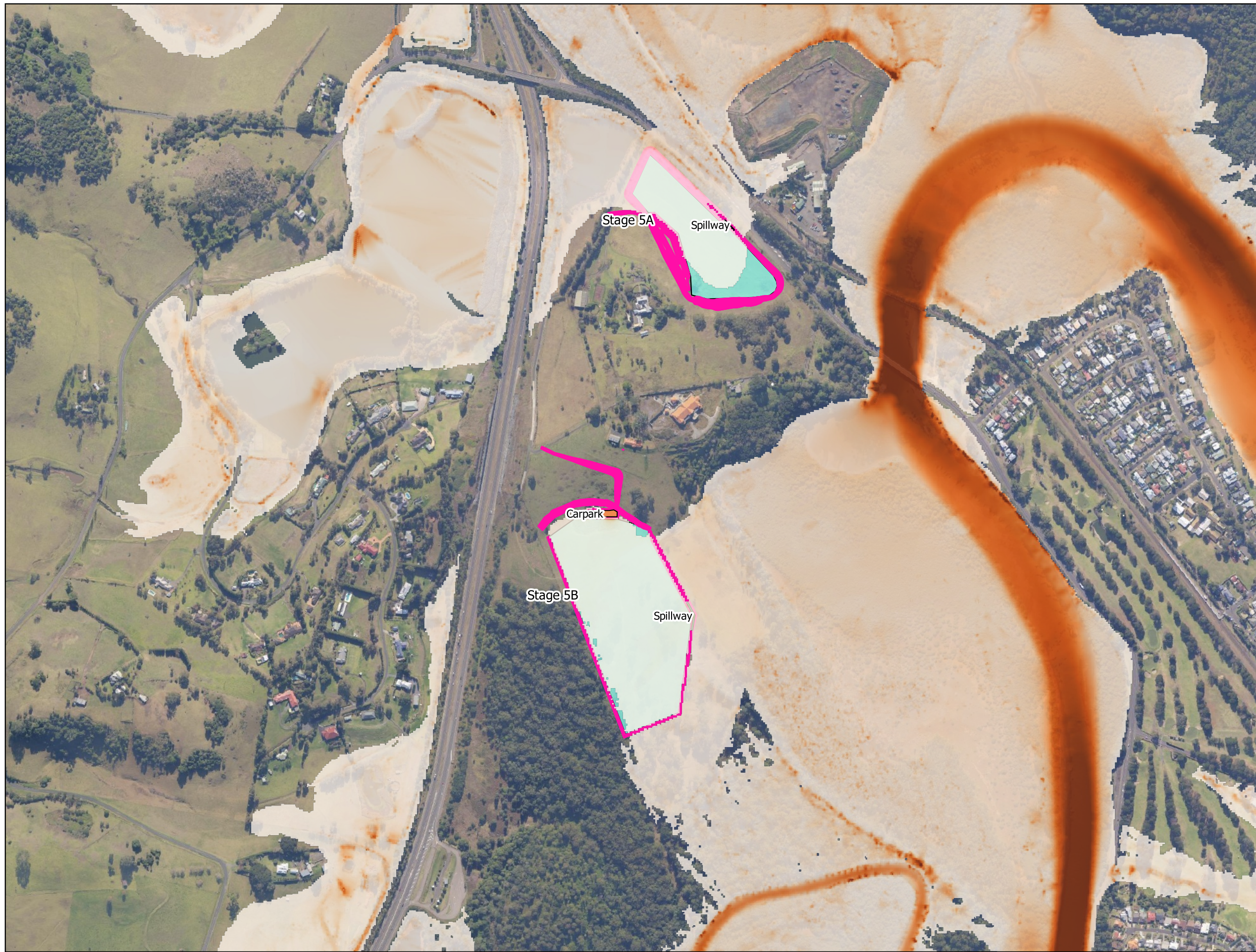
FIG 19. 100y ARI Max velocity, proposed conditions.
