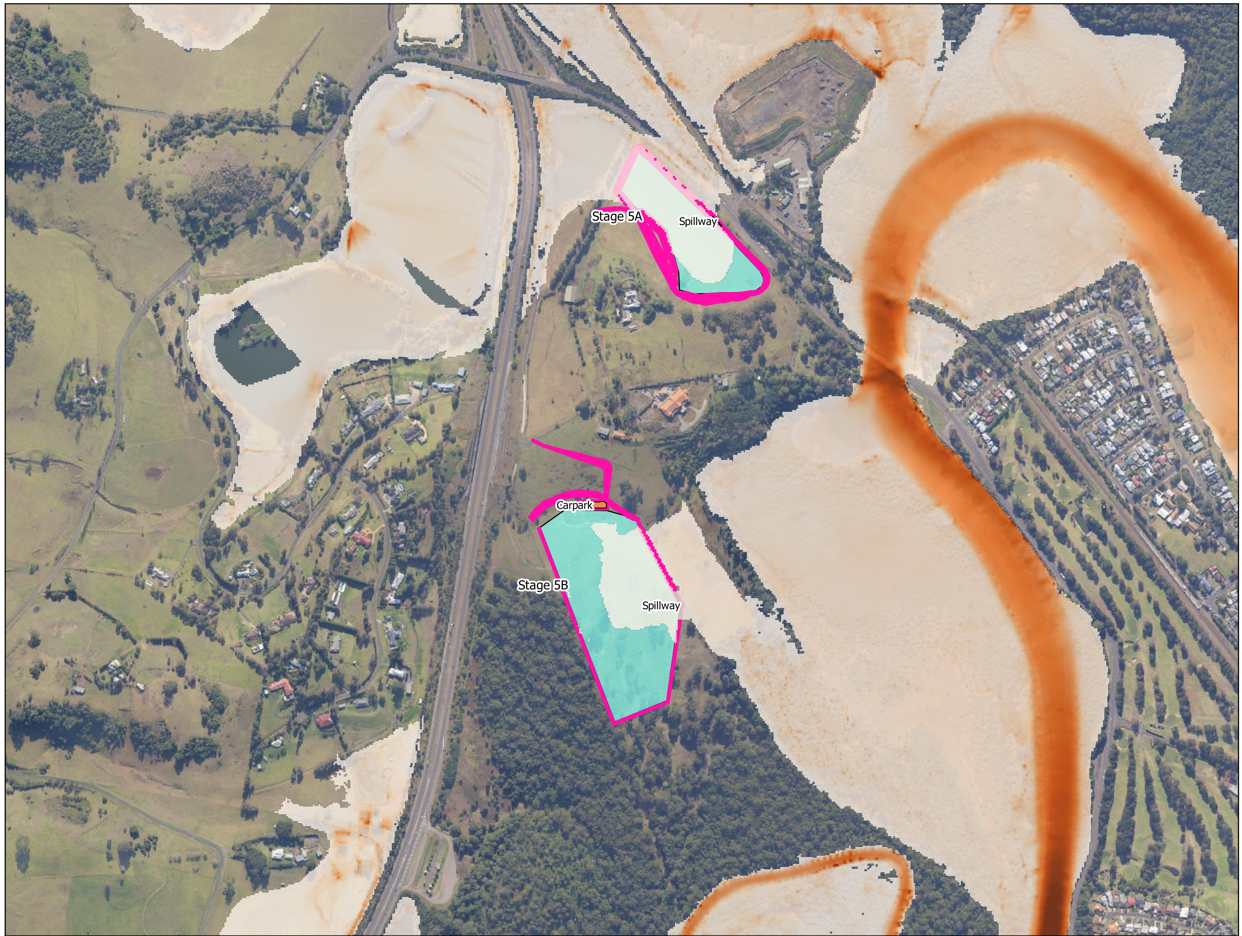
FIG 17. 5y ARI Max velocity, proposed conditions.
