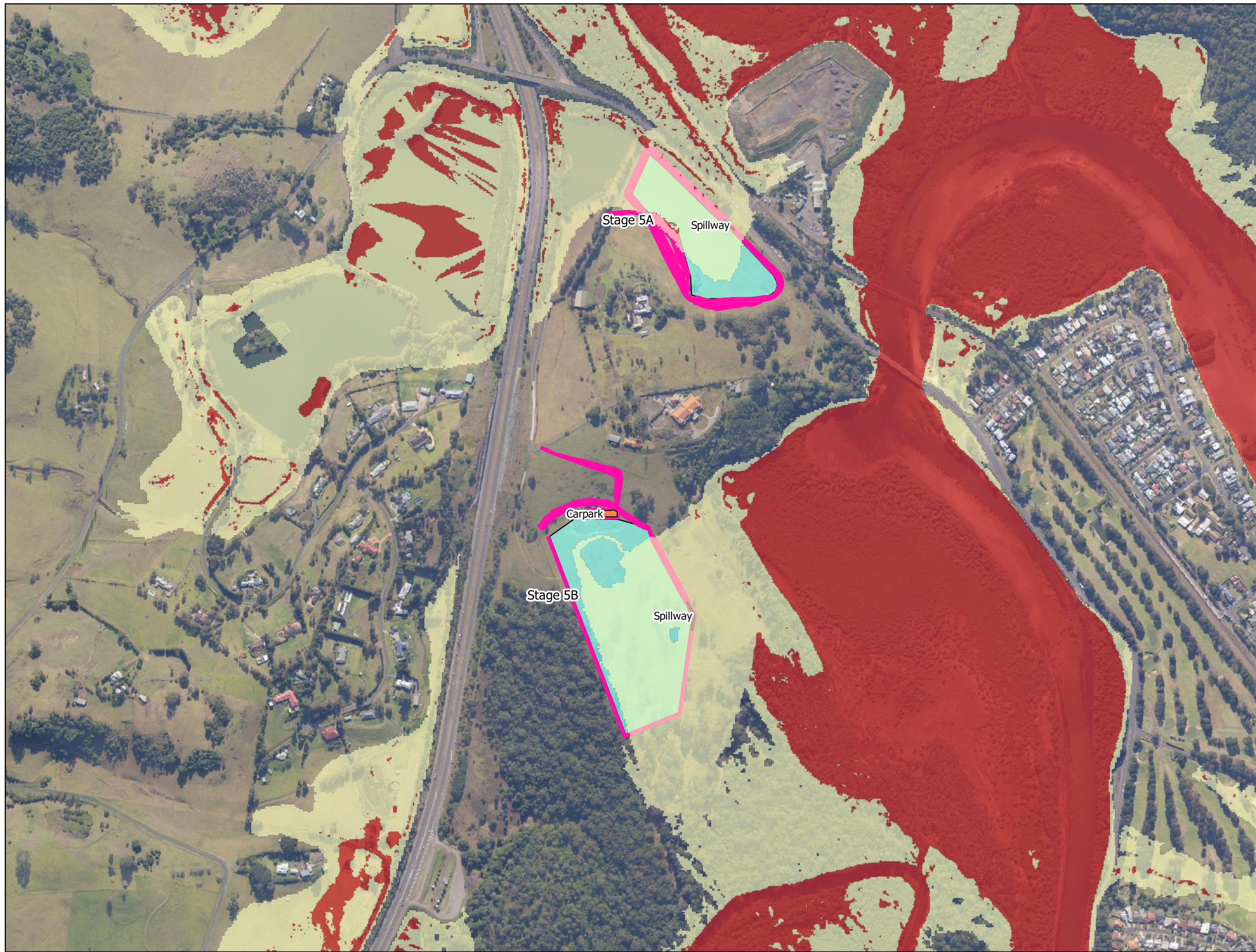
FIG 16. 100y ARI flood hazard, existing conditions.
