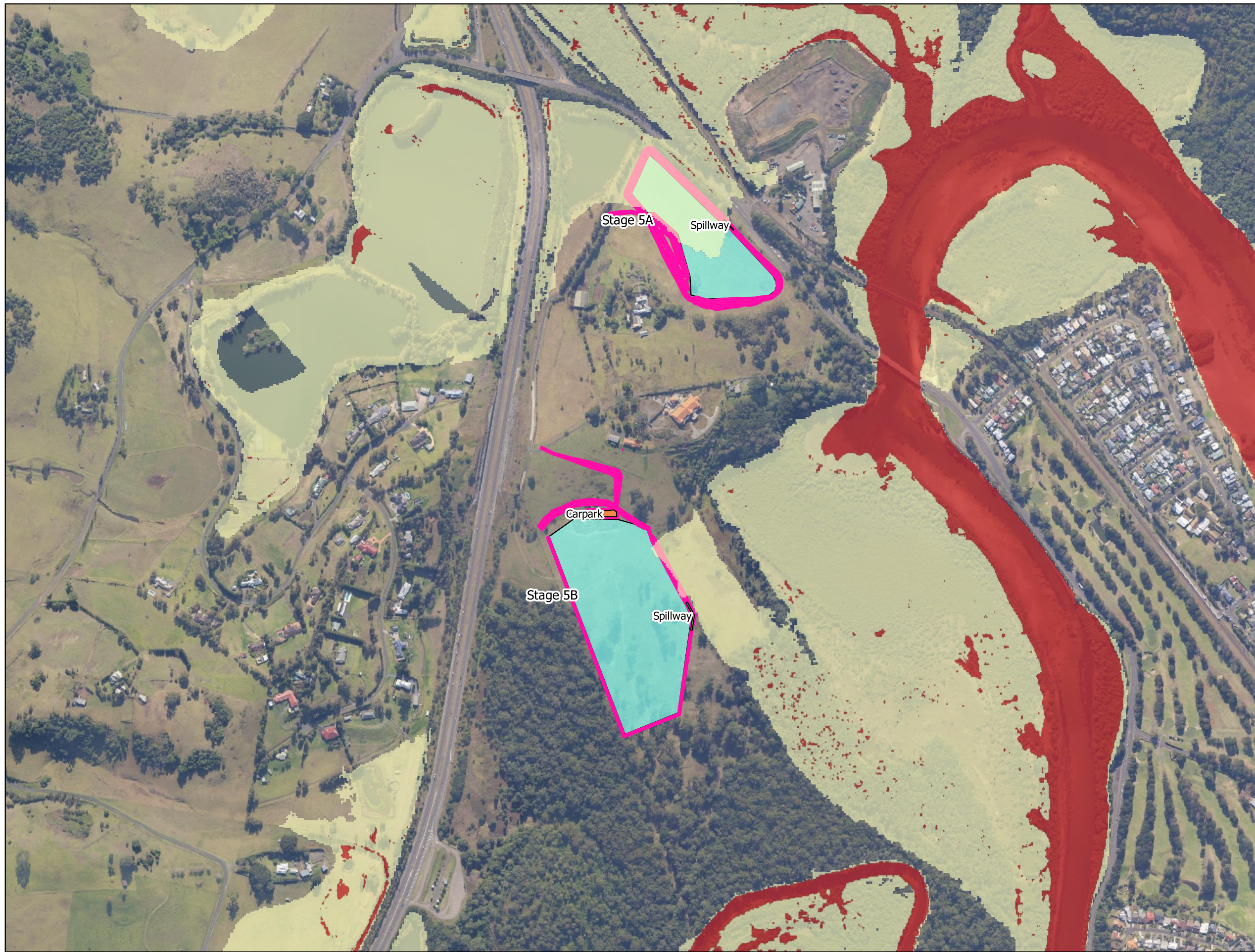
FIG 14. 5y ARI flood hazard, existing conditions. 18/07/2019
