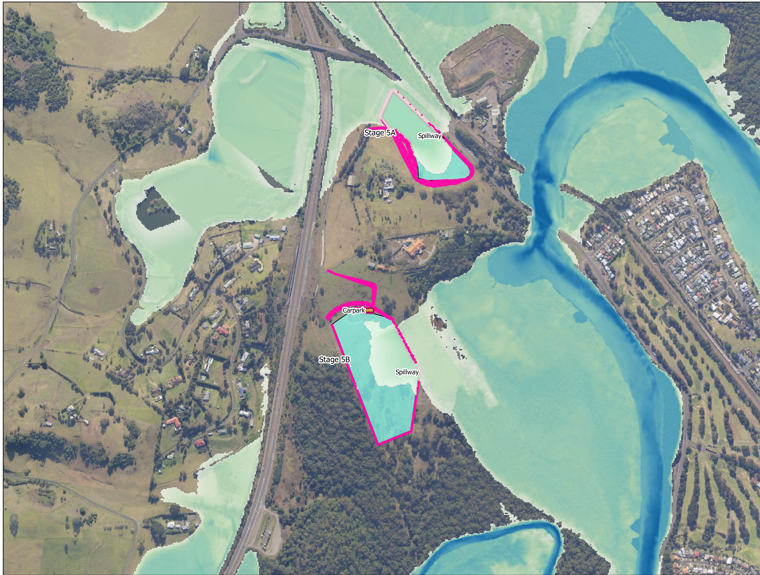
FIG 22. 20y ARI Flood depth, proposed conditions.
