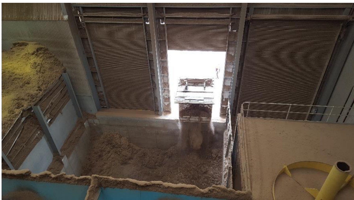
Plate 4 – Truck Vibrating to Discharge NSF into Receival Bunker
