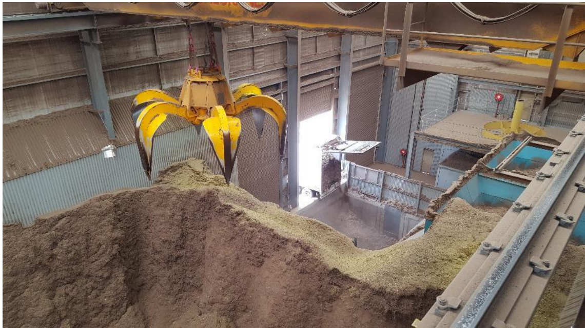
Plate 5 – Material Grab used to load conveyor system
