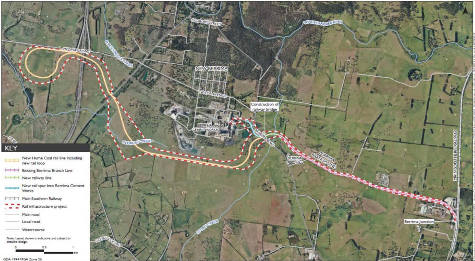
Figure 2.1: Extract from Hume Coal Berrima Rail Project EIS showing proposed rail route on the southern side of the Boral Cement Berrima Plant
