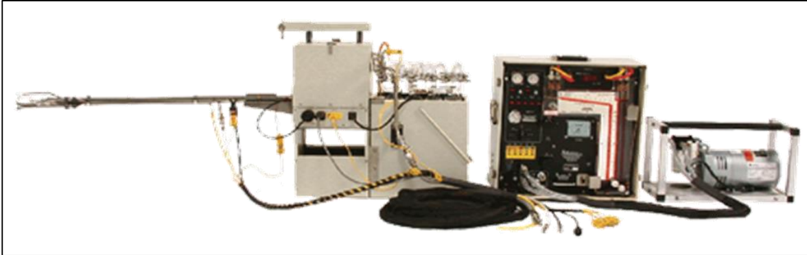
Figure 3: Full isokinetic sampling assembly
