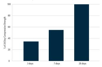
Cement Content = 320kg/m<sup>3</sup> Slump = 80mm
