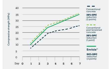
Field data (early-age strength will vary depending on the ambient temperature). The number of GBCA points are based on all mixes containing 50% recycled water and 25% manufactured sand.
