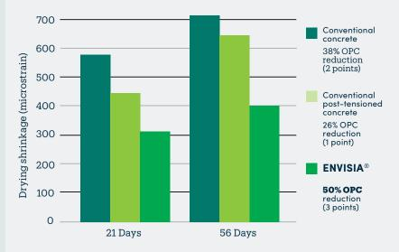
The number of GBCA points are based on all mixes containing 50% recycled water and 25% manufactured sand.
