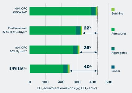
\* Based on the 40 MPa reference case in the Green Building Council of Australia rating tool \*\* Conventional 40 MPa concrete mixes
