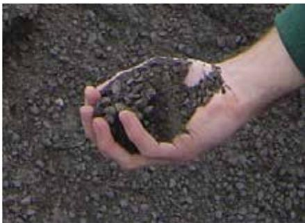
Processed reclaimed asphalt pavement (RAP).
