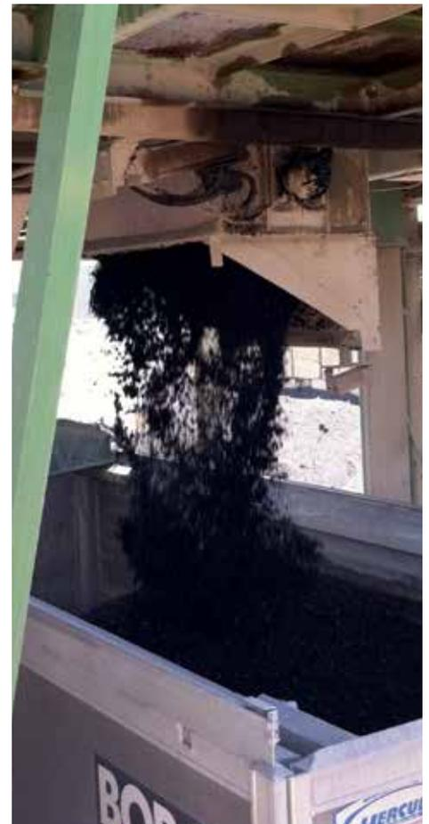
WarmPave asphalt being discharged into the tipper from the pug mill after mixing. Note the absence of any fumes.
