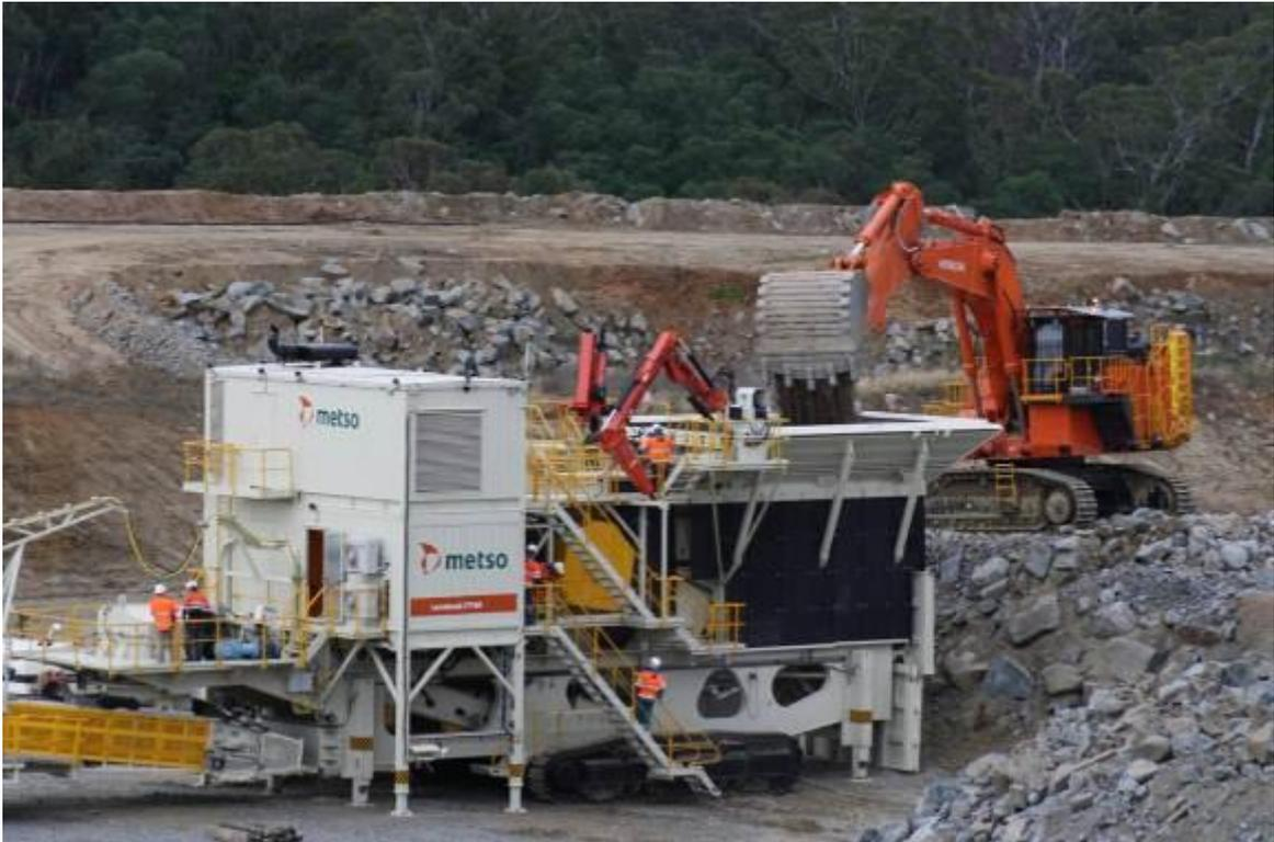
**Plate 6 – In-Pit Crusher in Operation**
