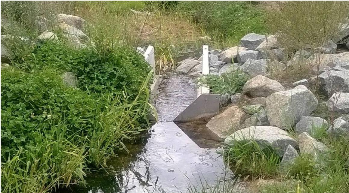
**Plate 10 - Water flow measurement in Tangarang Creek**
