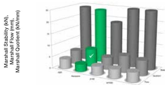
Fig6. Marshall Stability, Flow & Quotient
