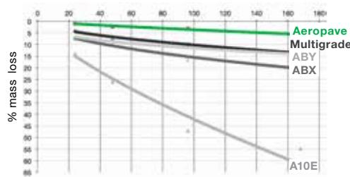
Fig2. Evaluation of Asphalt Fuel Resistance
