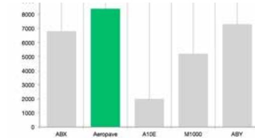
Fig5. Resilient Modulus (MPa)
