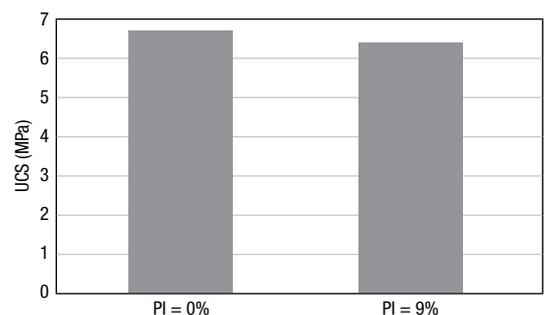
*Note: Test method used - RMS T131 7 Day Accelerated (AC) UCS. (Samples @ 1 hour after mixing binder)*
