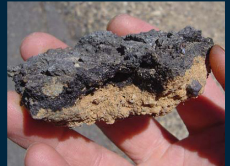
The penetration of GATT binder into the gravel base course.
