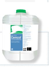
Boral Cements Blue Circle® Cemcol is a clear liquid air entraining agent that creates small bubbles of air throughout the mix and improves workability in cement based brick mortars and renders.
