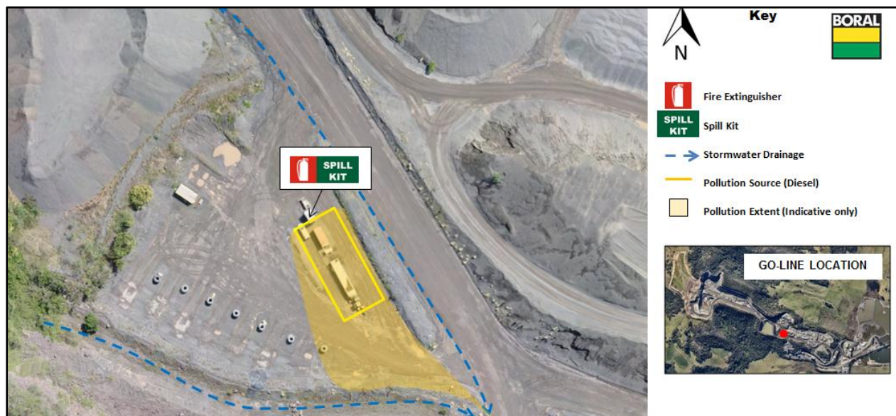
Figure 3: Go-line Above Ground Diesel Storage Area
