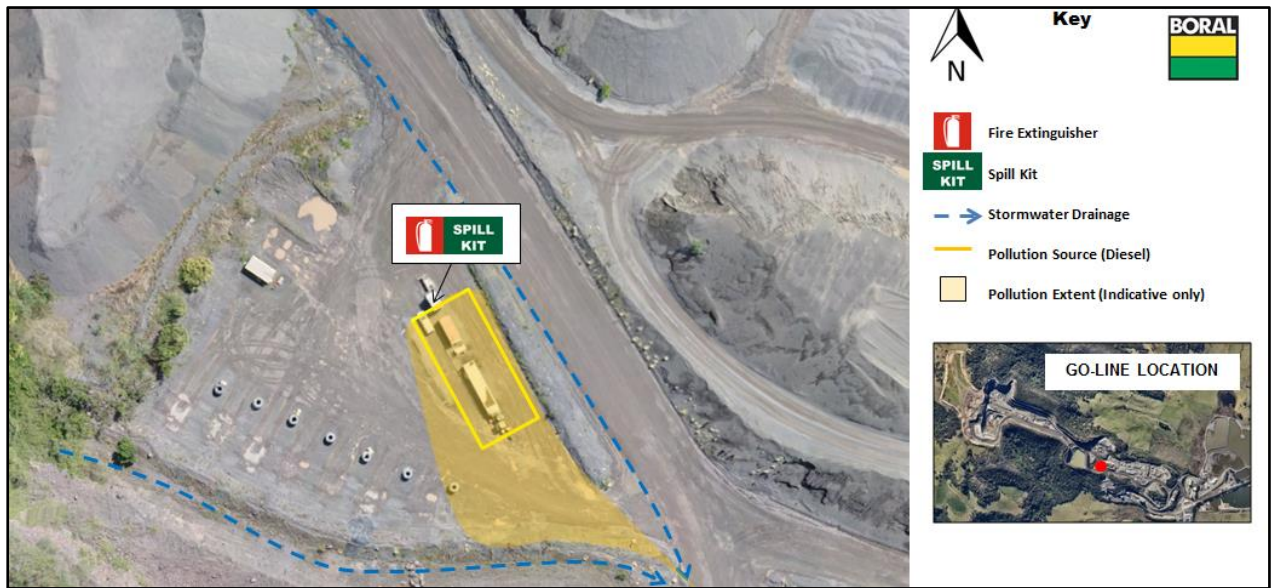
Figure 3: Go-line Above Ground Diesel Storage Area
