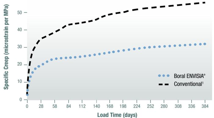
Note: Conventional<sup>1</sup> concrete = standard concrete with same aggregates as ENVISIA® but with 84% SL cement and 16% Fly ash.
