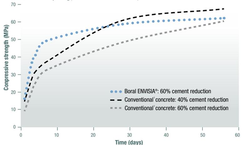
Note: These are 40 MPa concretes typical for post-tensioned construction. Stressing times increase for conventional¹ concrete as the cement reduction level increases. Cement reduction calculated using Green Star 'MAT-4' method.
