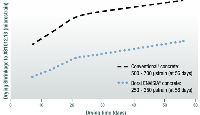
Note: These are typical results based on 40 MPa grade concrete. Shrinkage will vary according to the specific aggregates used.
