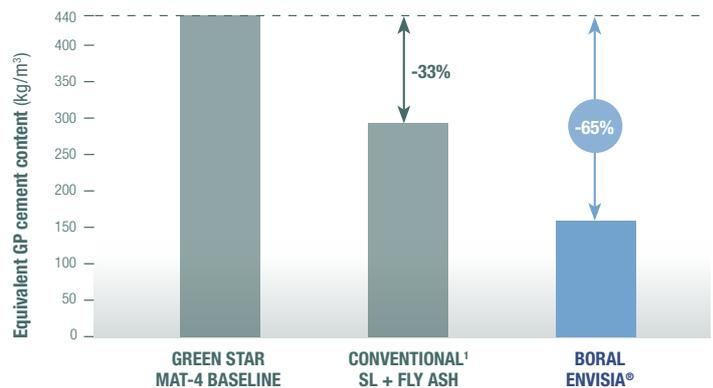
Note: This is for 40 MPa post-tensioned concrete and comparison based on the Green Building Council of Australia material credit for concrete MAT-4.<sup>^</sup>
