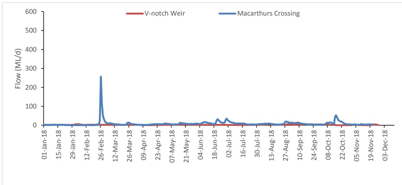
Figure 2: River flow at Wingecarribee River - Medway and V-notch weir (January 2018 - October 2018)
