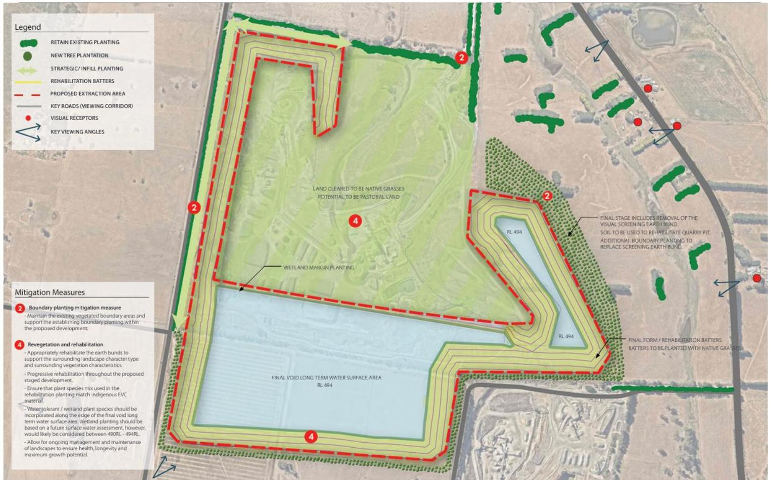
Figure 2: Final stage rehabilitation framework plan
