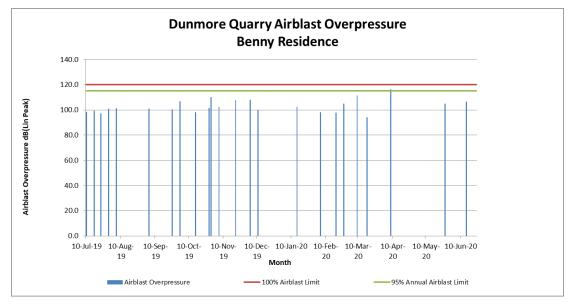
Figure 12 current reporting period Airblast Overpressure Monitoring Data
