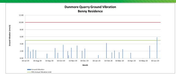
Figure 13 FY20 Ground Vibration Monitoring Data
