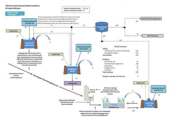
Figure 31 Existing Water Management System Typical Dry Year Water Balance
