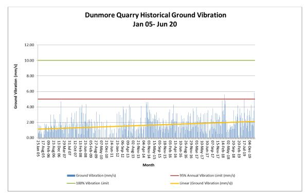
A visual representation of historical blast monitoring data can be seen below in Figure 14 and 15.
