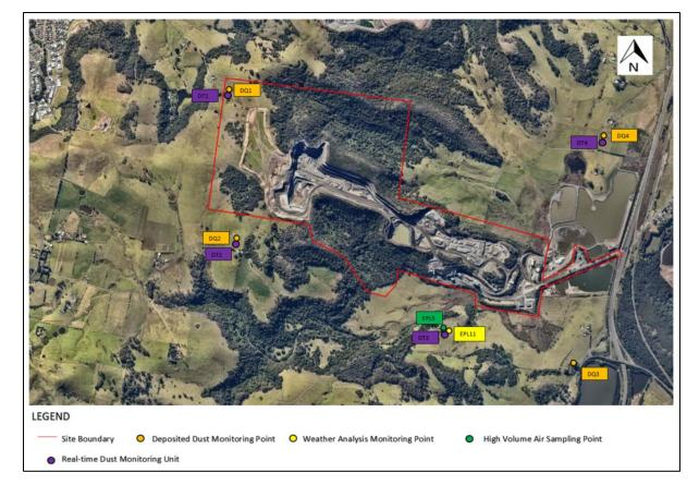
The location of the DQ air quality monitoring equipment is shown below in Figure 2.
