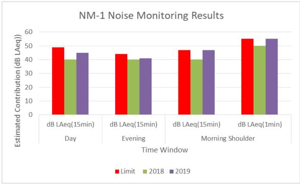
Figure 18 Post MOD 9 NM-1 Noise Monitoring Data
