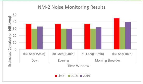
Figure 19 Post MOD 9 NM-2 Noise Monitoring Data
