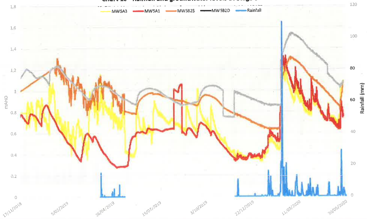
Chart 1c - Rainfall and groundwater levels at Stage 5
