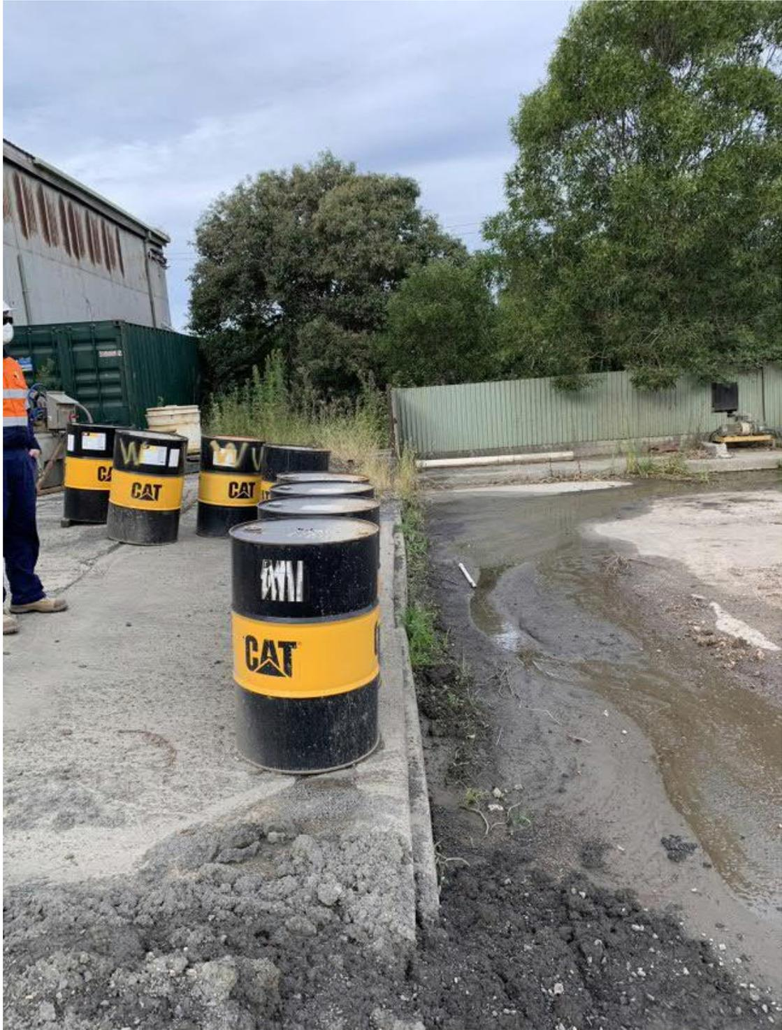
**Oil drums being incorrectly stored outside appropriately bunded area.**
