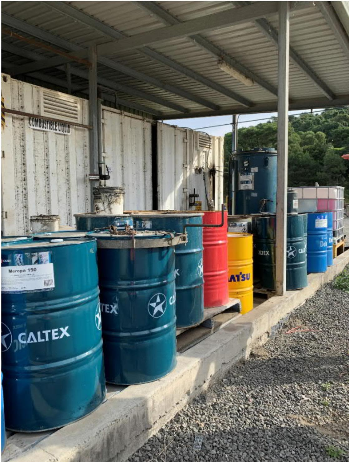
Oil drums being incorrectly stored, overhanging bunded area near maintenance workshop.
