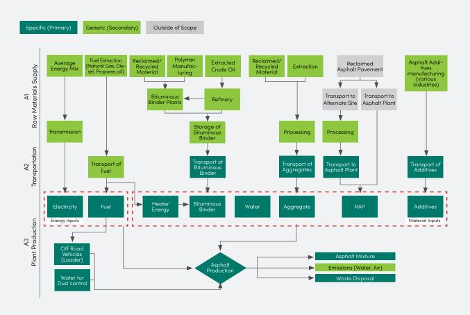
Above: Flow diagram of asphalt production process (life cycle stages A1 to A3), data types and system boundaries (AEPDP 2019)
