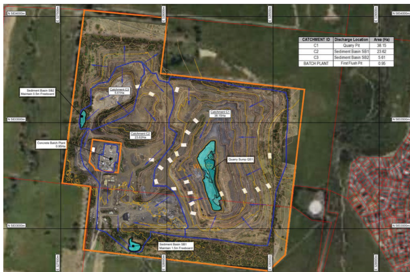
Figure 3 Surface Water Management
