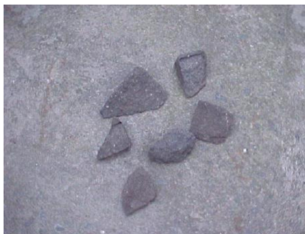
Photo 5 – Old Train Block Fragments containing Asbestos
