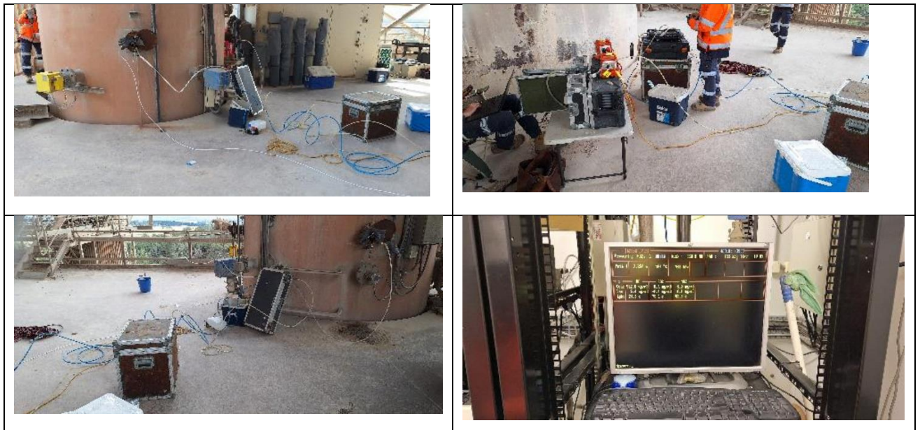
Plate 5 – Ektimo Equipment undertaking 6 monthly Stack Emission Verification Testing
