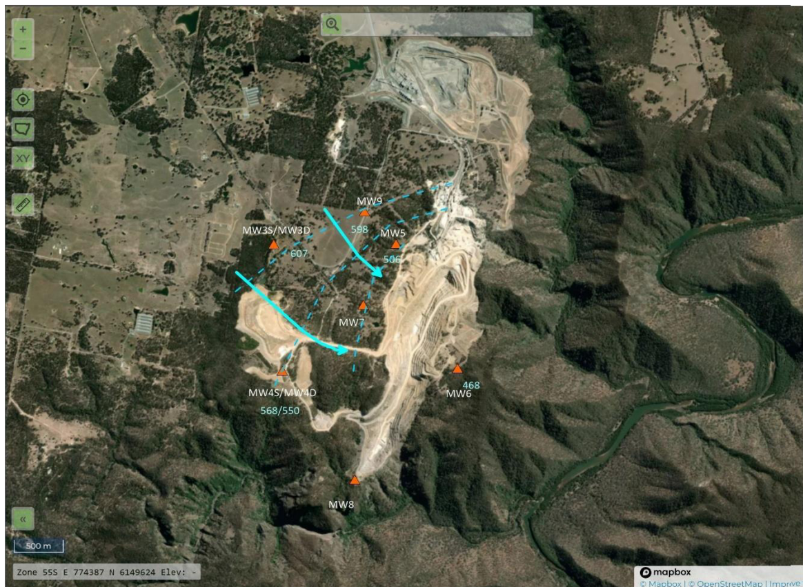
Figure 10 Map with piezometric levels (2025) , interpreted contours (blue dotted) and flow direction (blue arrows)
