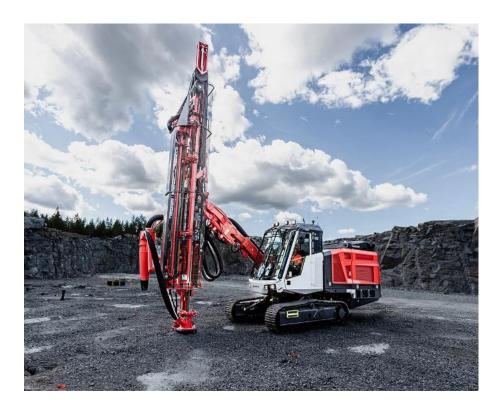
A hydraulic, diesel-powered, self-propelled top hammer drill rig. Designed for large hole drilling, it is suited to production drilling in large quarries or open pit mines.
