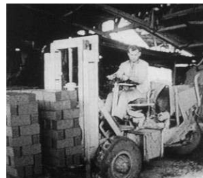
Dominic Stante on a forklift modified from a Bren gun carrier.
