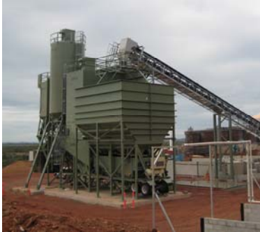
High capacity mobile concrete plant purchased for Gladstone smelter upgrade
